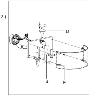
Step2:Wire fixture to wires in outlet box.
