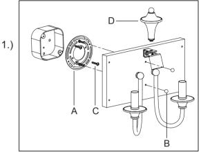
Step1:Remove mounting bracket from fixture and install to electrical box.
