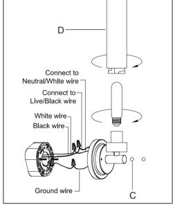
Step2:Wire fixture to wires in outlet box. Copper wire is for Ground. Attach canopy to mounting bracket and tighten with ball nuts.
