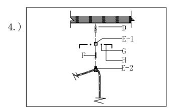
Step. 4: Install Wall plug(D) into the ceiling, And use the tapping screw(F) to lock the wire holder cap(E-1). Then install wire holder (E-2) into cap, and use wrench(F) to tighten screw(G) to lock wire holder in the cap.
