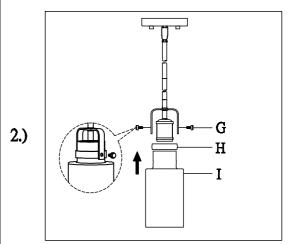
Step.2: Attach metal ring (H) and glass (I) to yoke and secure using set screws(G).
