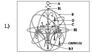
Step.2: Hang the crystal (CRP032/2J) on the metal cup(B2) Put the tube(C) onto the metal cup(B2) Locked the loop(A) to the nipple(B1) till tighten
