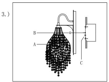
Step. 3: Attach fixture to mounting
