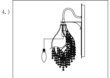
Step. 4: Install max 60 watt candelabra bulb (not included) into socket.
