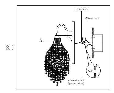
Step. 2: Carefully unwrap fixture. Wire fixture to wires in outlet box. Copper/green wire is for Ground.
